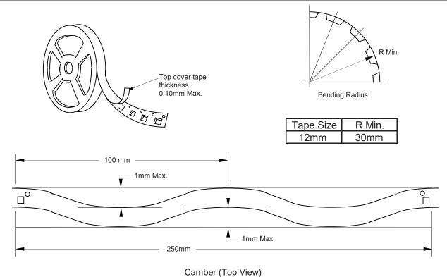
Allowable camber to be 1mm/100mm non-accumulative over 250mm
