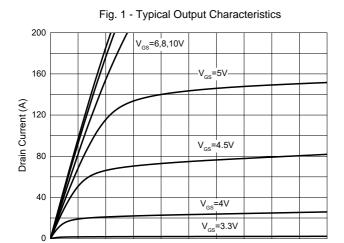
Drain To Source Voltage (V)
